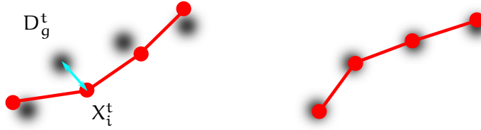
Figure 5.2: The observation model minimizes the distance between the detections (gray blobs) and the estimated trajectories.
