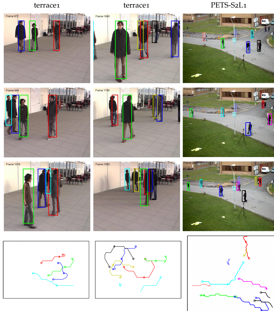
Figure 4.6: Tracking results obtained with the proposed ILP algorithm. The left and middle columns are from the terrace1 sequence, the right column is from PETS-S2L1 . Displayed are three sample frames (1 st -3 rd row), and a bird's-eye view of target trajectories (last row). The displayed frames are marked (top \circ , middle \diamond , bottom \square ). See Section 4.4.1 for details.
