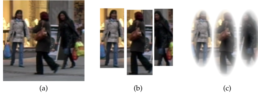
Figure 5.11: Instead of extracting and comparing full bounding boxes (b), we propose to weigh the area using anisotropic Gaussians (c). The energy remains differentiable, and the influence of undesired background pixels is reduced.
