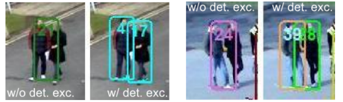
Fig. 8. Influence of the detection-level exclusion term E_{\text{det}}^X , which prevents that two separate targets are assigned the same ID.
