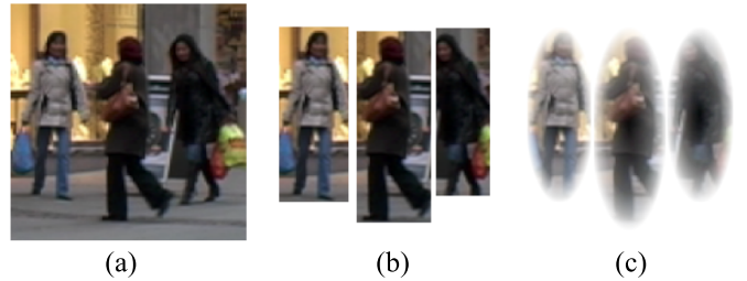
Fig. 5. Instead of extracting and comparing full bounding boxes (b), we propose to weigh the area using anisotropic Gaussians (c). The energy remains differentiable, and the influence of undesired background pixels is reduced.
