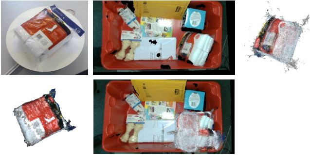
Fig. 8. Pose registration. Left column: Turntable capture, resulting model. Center column: Scene, scene with initializations. Right column: Final registered model.
