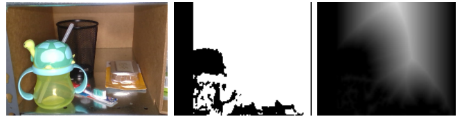
Fig. 12. Retract planning. Left: RGB image of the scene. Center: Front-projected collision mask for retrieval of the black pencil cup. The sippy cup is not fully masked because of missing depth values on the transparent surface. Right: Distance transform.
