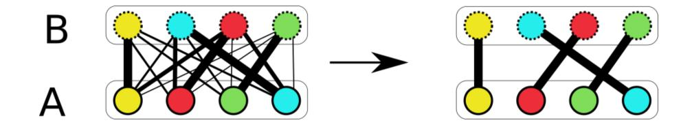
Linear Assignment:  $X^* = \underset{X}{\operatorname{argmin}} \quad C^\top X$  s.t. X binary and one-to-one
